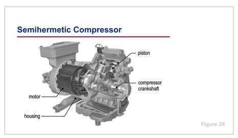
Similarly, the motor for a **semihermetic compressor** is also contained within the compressor housing and is cooled by the refrigerant. The term "semihermetic" means that the sealed housing is designed to be opened to repair or overhaul the compressor or motor.
